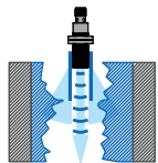
Figure 6 - Applying Ultrasonic Sensor
